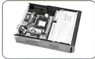
10: Cages on the screw 5"25 revolving to the rack, and installs VGA card
