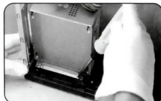
2: Remove 2pcs screw, take down power supply
