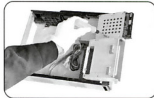
7: Installs the hard disk
