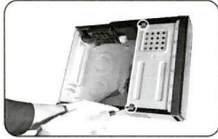
2: Lies the case on the tabletop Twists off two screws on the 5"25 bay
